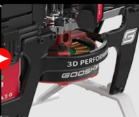
Figure 2.2.5: Flight Control, ESC, and Motor Components. This image highlights the brand-new flight control design with ELRS protocol support, the split-type ESC, and the newly designed high power density motor, offering a 20% increase in power output.
