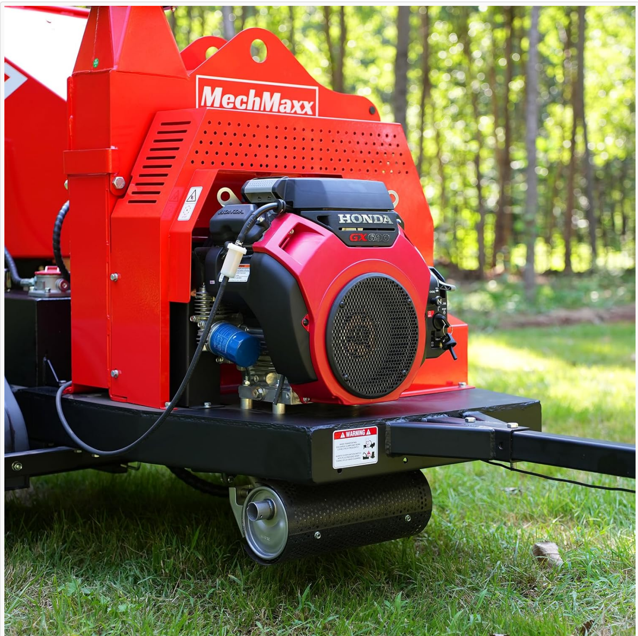
Image 3.2: Close-up view of the Honda GX690 engine, highlighting its placement on the chipper.
