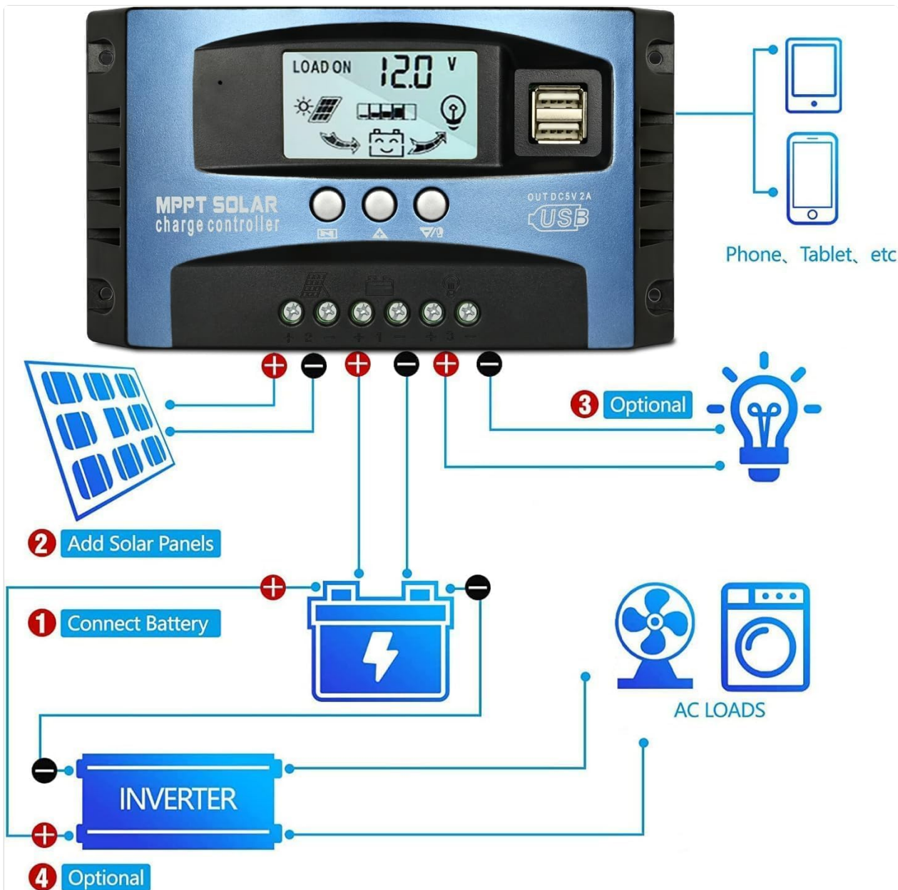
Figure 7: Connection diagram for the 100A MPPT Solar Charge Controller. Follow the numbered sequence for installation.
