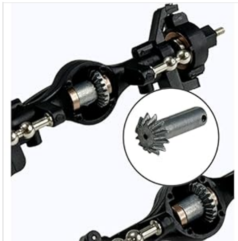
Figure 7: Detail of the solid axle and differential gear.
