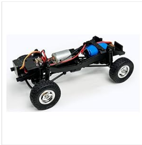
Figure 6: Internal chassis view showing motor, ESC, and battery placement.
