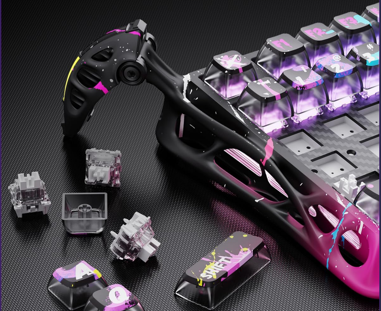
Figure 8: Hot-swappable design for easy customization.
