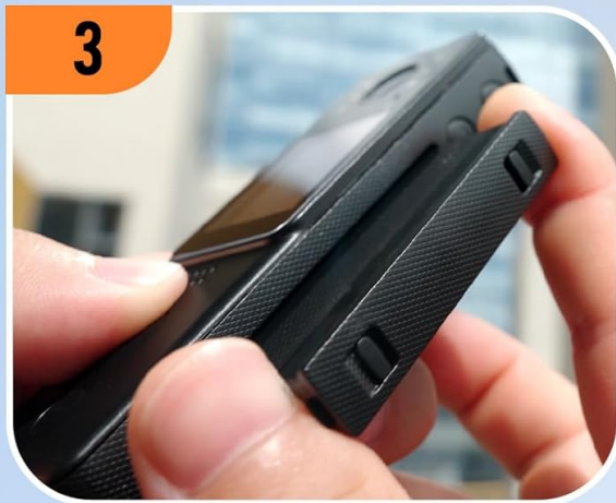
Figure 2: Replacing the Losfom Z11 battery. Press the latch, pop out the battery, and insert a new one.
