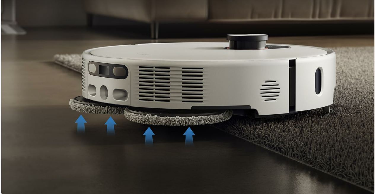
Figure 6: Ultrasonic carpet detection system, which automatically lifts mop pads by 15mm to avoid wetting carpets, offering multiple cleaning modes.
