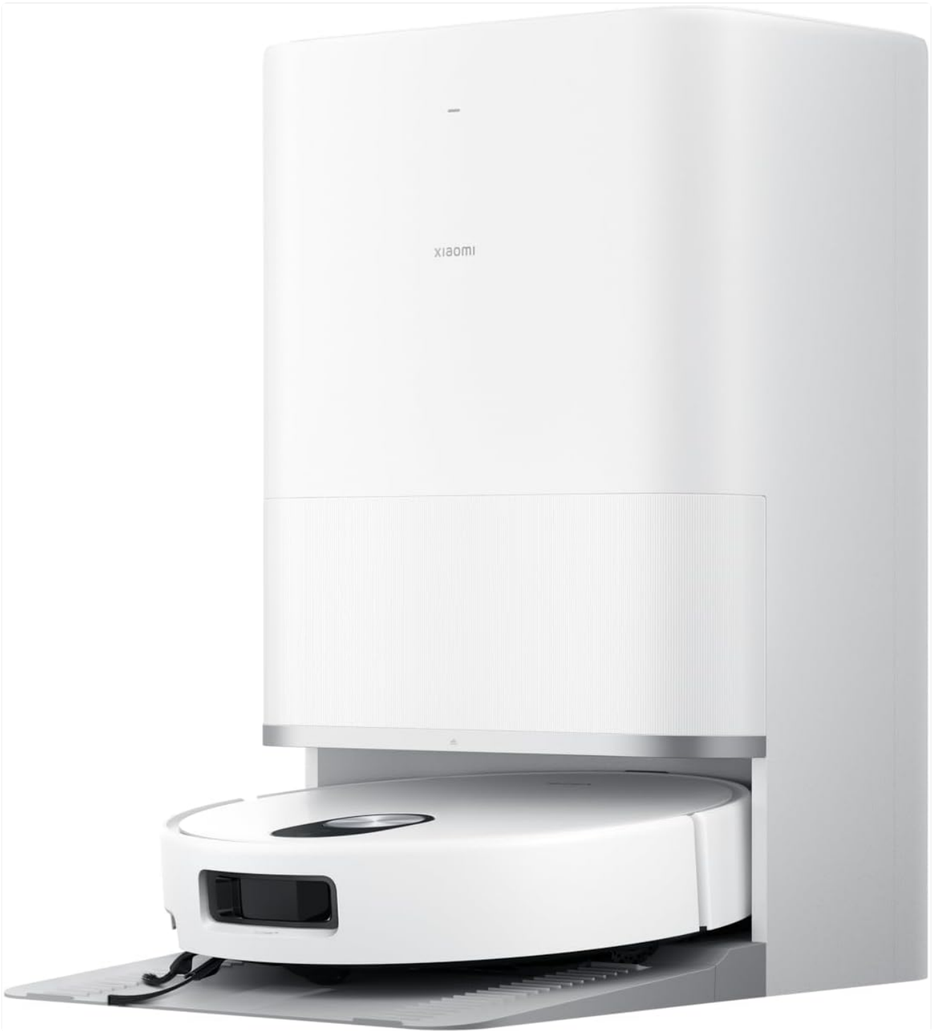
Figure 3: The robot vacuum docking with its base station for charging and self-cleaning.
