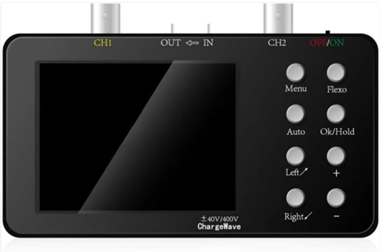
Figure 2.1: Front view of the SCO2 Dual Channel Digital Oscilloscope, showing the display and control buttons.
