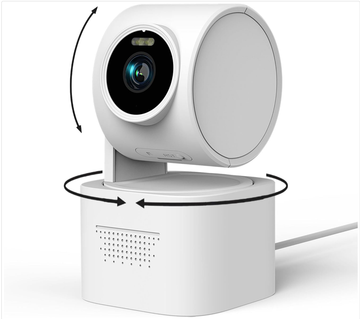
Figure 2.1: Girafit GRF-T350SW camera showing its pan and tilt capabilities.
