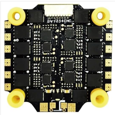
Top view of the ZTW 60A 4-in-1 ESC board, highlighting the large soldering pads and component layout.
