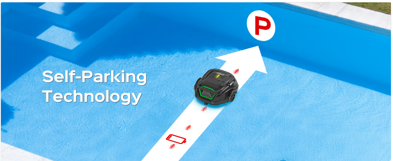
The WYBOT A1 demonstrating its self-parking technology, returning to the pool edge when its battery is low for easy retrieval.
