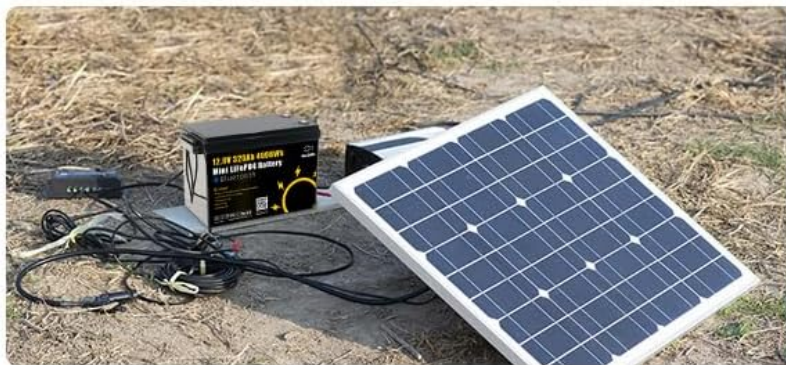
Figure 5.1: Three ways to recharge the battery. This image illustrates different charging methods: using a generator, a dedicated charger, or a solar panel with an MPPT controller.
