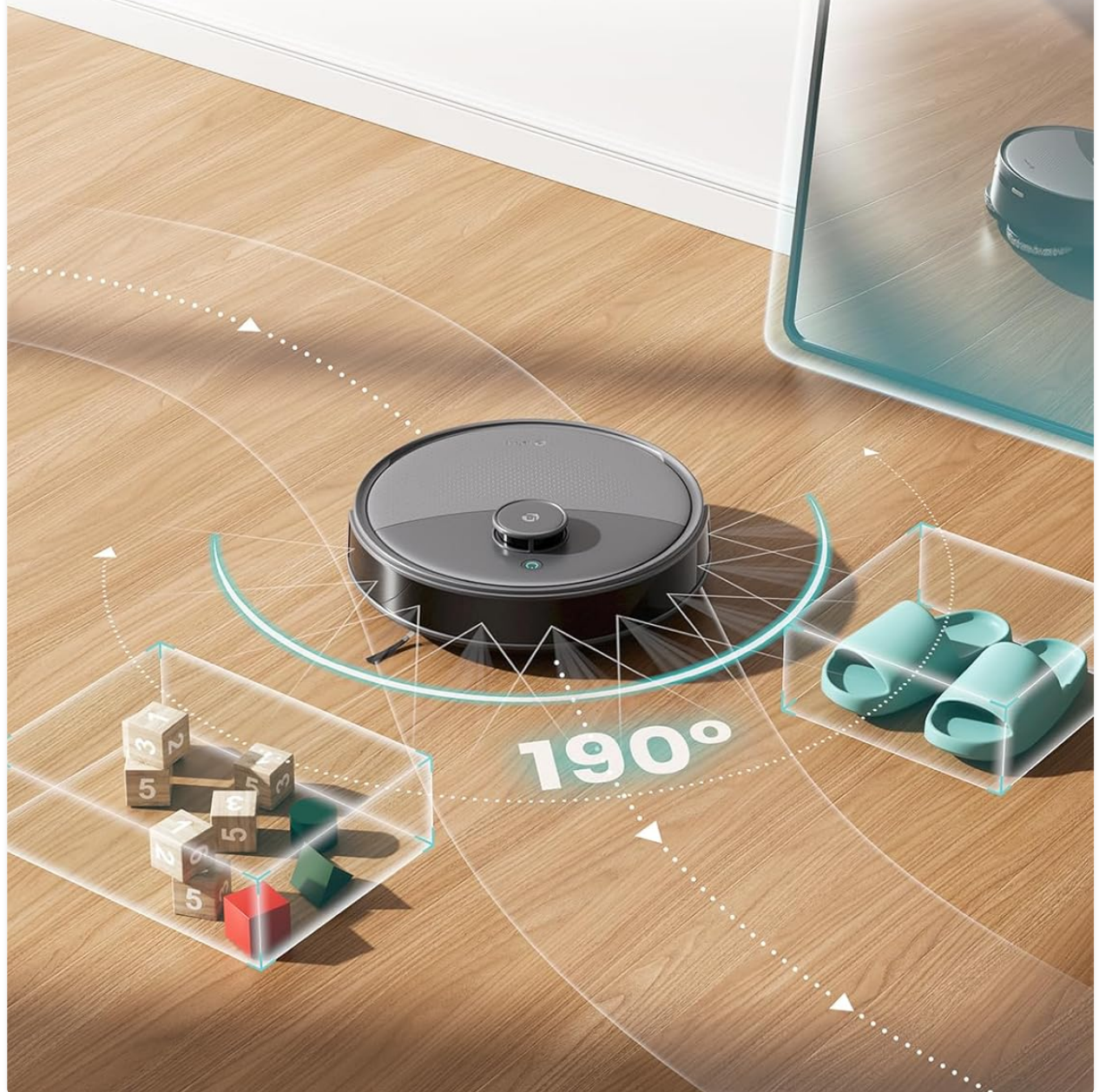
Image: The robot detecting and avoiding various objects on the floor using its 190° PSD sensors.
