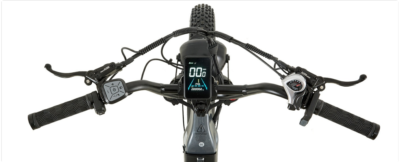
Figure 3.1: Handlebar assembly with the integrated LCD display and control buttons.
