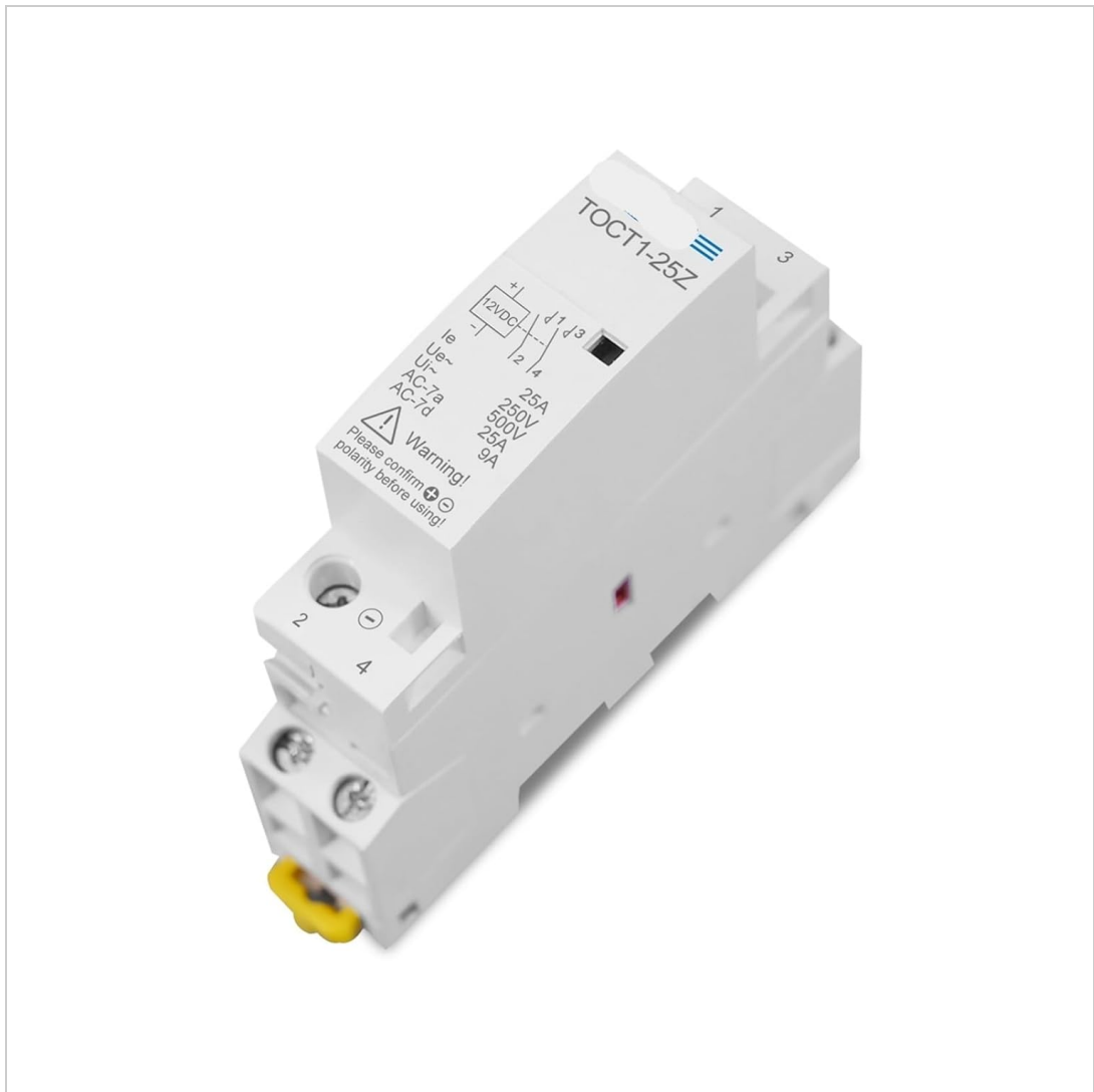
Image: A close-up view of the TOCT1-25Z contactor, highlighting the 12VDC coil input terminals and the internal wiring diagram. A warning about confirming polarity is visible.
