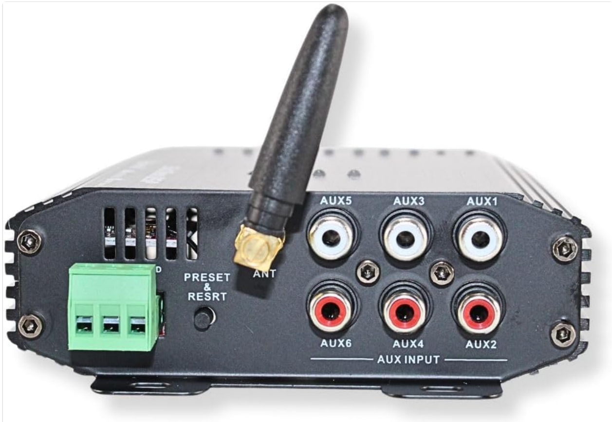
Image: Front panel of the DSP, illustrating the RCA input connections (AUX1-AUX6) and the power terminal block.
