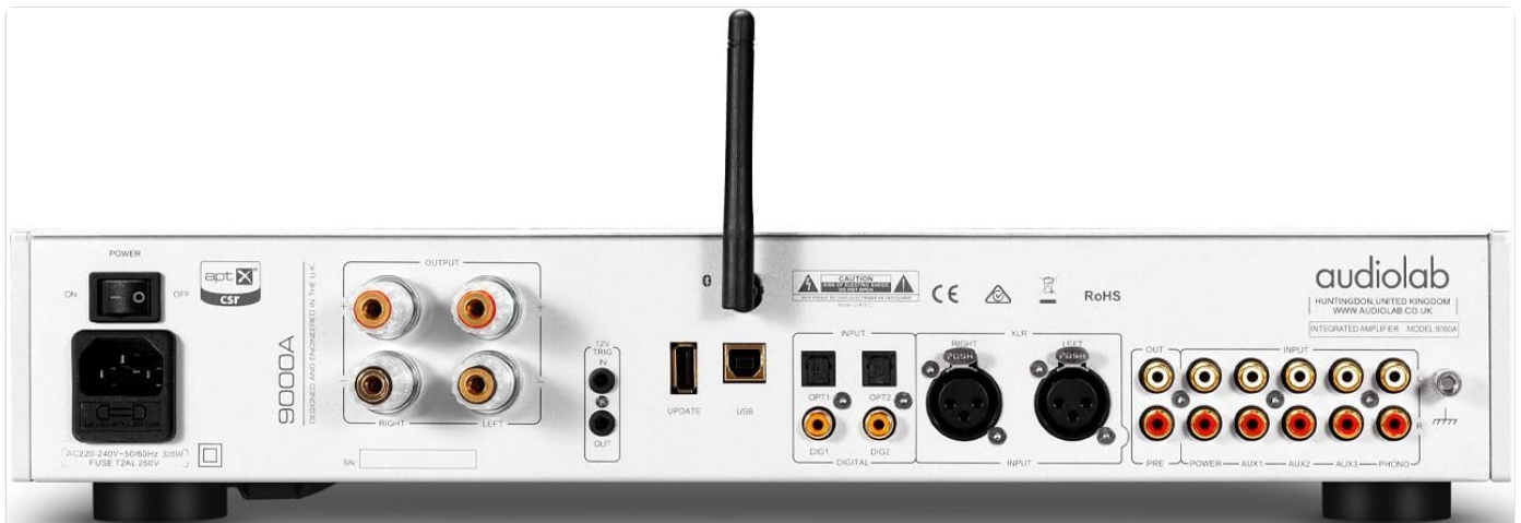
Figure 4.3: Rear panel of the Audiolab 9000A, showing a comprehensive array of input and output connections. These include analog, XLR, phono (MM), power amplifier input, SPDIF (coaxial and optical), PC USB, Bluetooth antenna, pre-amplifier output, stereo speaker terminals, and 12V trigger connections.
