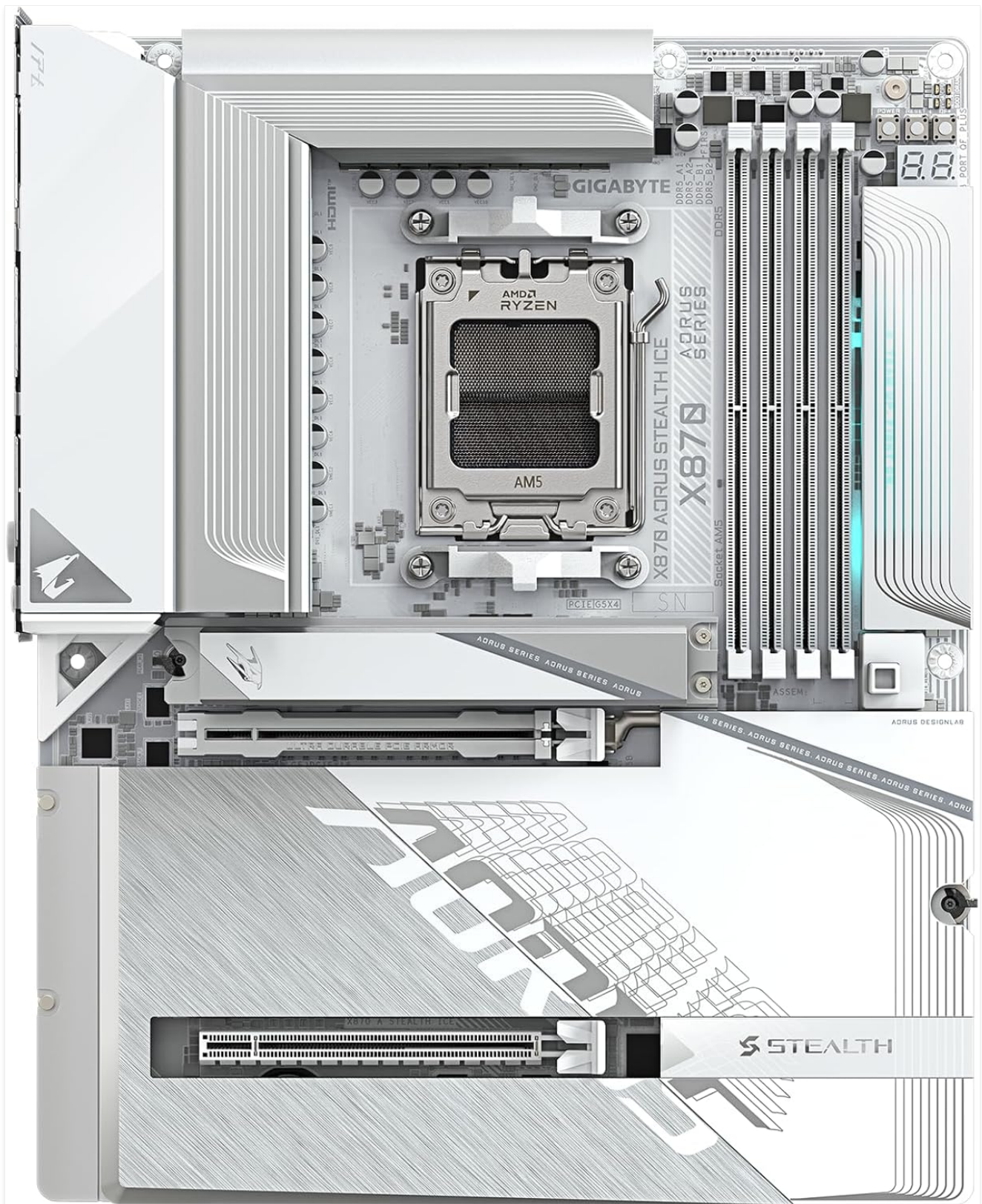
Image 2.1: Top-down view of the GIGABYTE X870 AORUS Stealth ICE motherboard, highlighting the CPU socket, DDR5 RAM slots, and M.2 slots.
