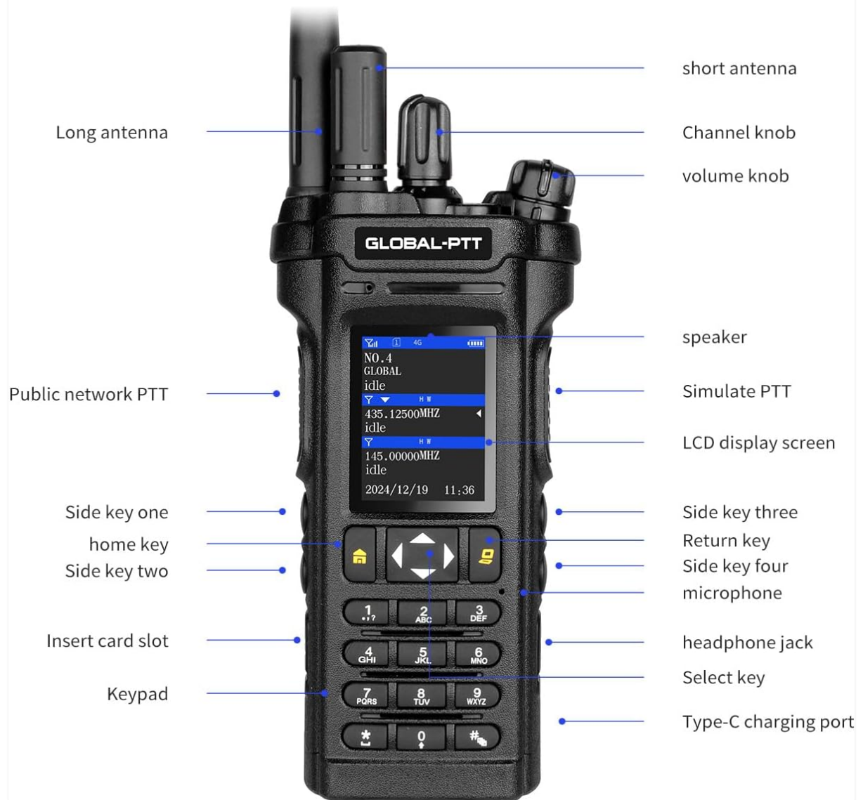
Image: A detailed view of the GLOBAL-PTT 5288 Plus radio, highlighting and labeling its various function keys, knobs, ports, and display screen.
