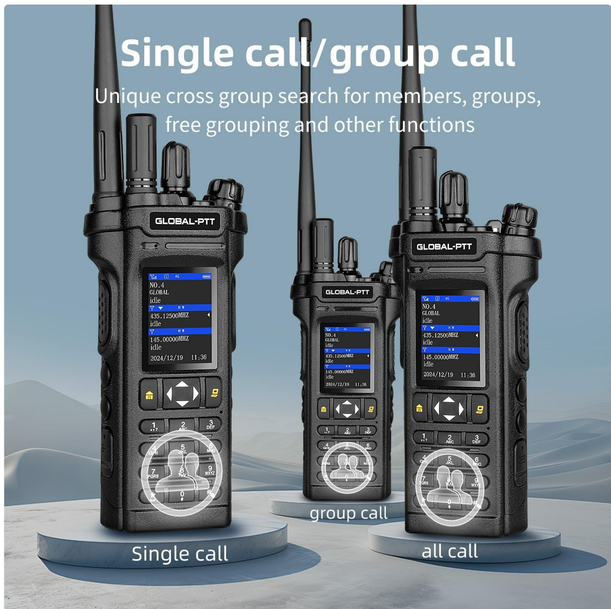
Image: Three GLOBAL-PTT 5288 Plus radios arranged to show the concepts of single call, group call, and all call communication modes.
