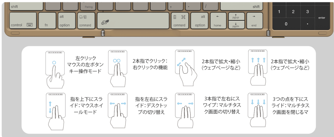
Image: Illustration of the touchpad and numeric keypad functionality, highlighting the toggle feature.
