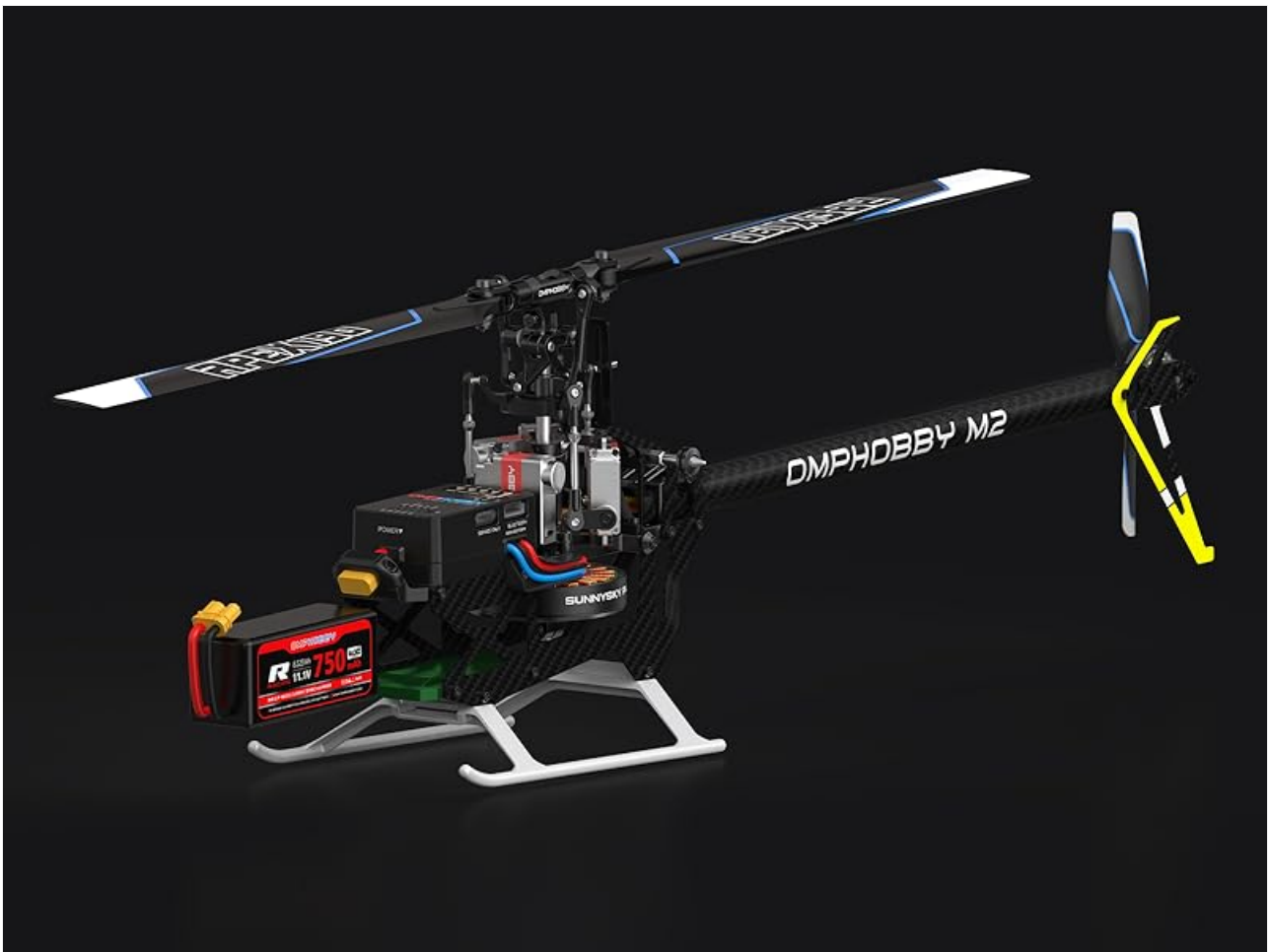
Figure 5.1: Battery installation on the M2 V3 PRO.
