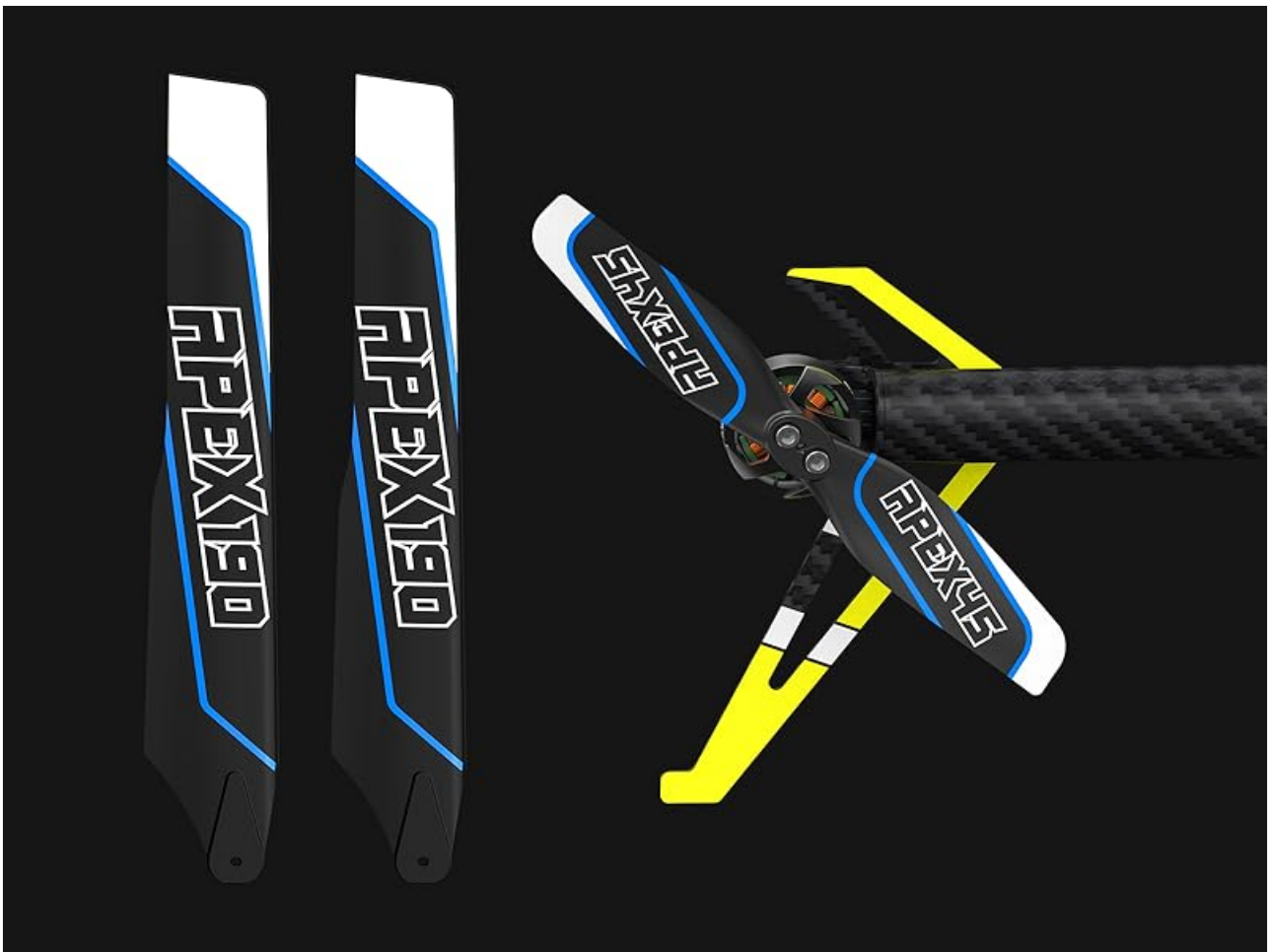
Figure 8.1: Main and tail rotor blades.
