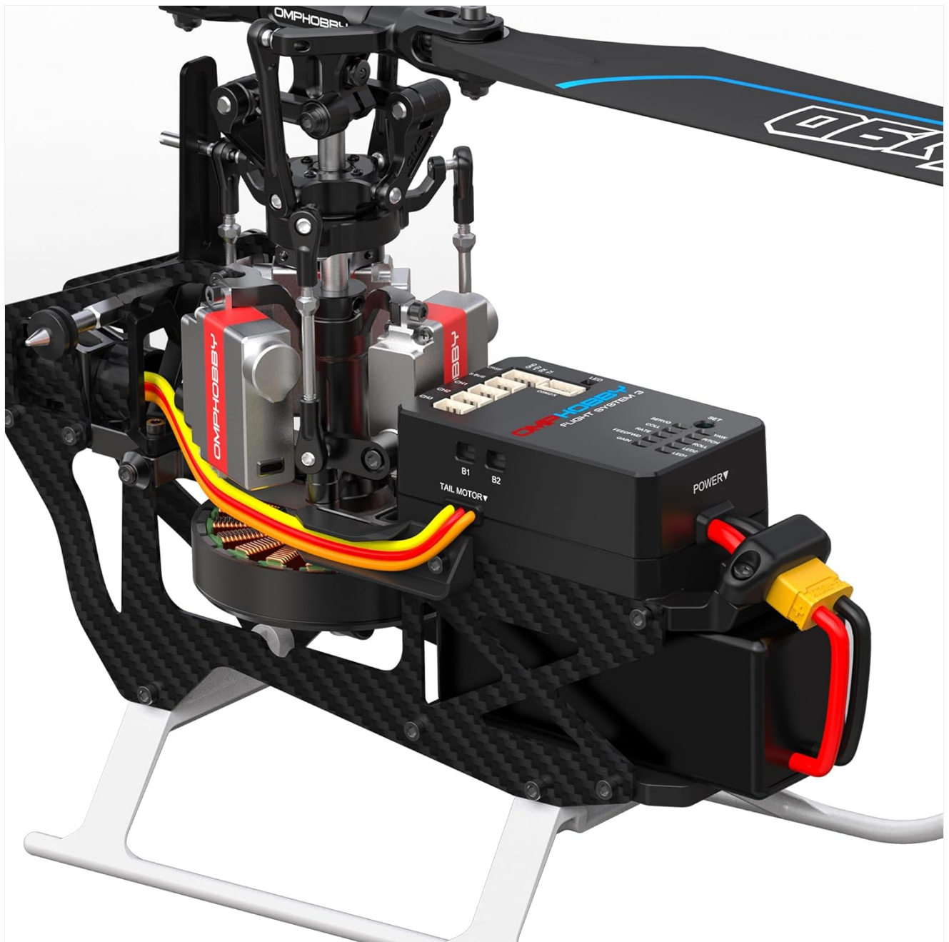
A detailed view of the internal components, including the flight controller and brushless motors.
