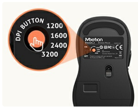
Image: A close-up of the mouse's underside, showing the DPI button and its corresponding sensitivity levels.
