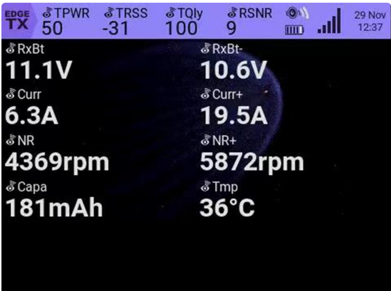
Image: A close-up of a radio transmitter screen showing real-time telemetry data, including receiver battery voltage (RxBt), current (Curr), rotor RPM (NR), battery capacity used (Capa), and temperature (Tmp), providing critical flight information.
