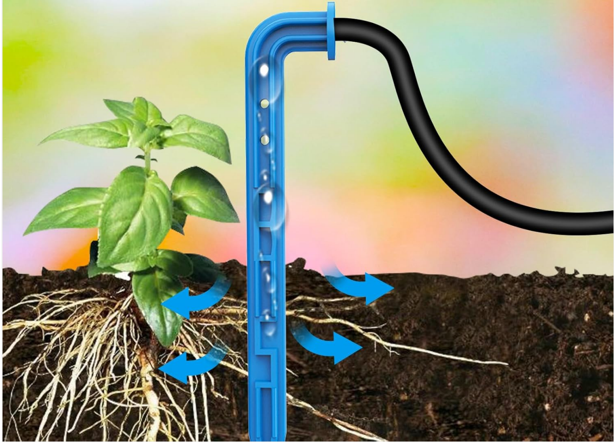
Image: Deep drip irrigation system delivering water directly to the root zone of a plant.
