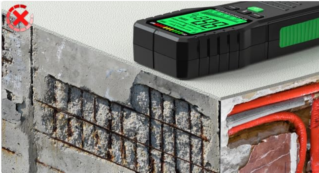
Figure 5: Incorrect usage of the moisture meter, demonstrating how metal objects like rebar and pipes can interfere with readings.
