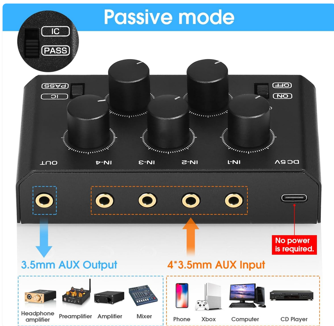
Figure 4.3: The rear panel of the mixer showing four 3.5mm AUX input jacks, one 3.5mm AUX output jack, and a USB-C port for optional 5V DC power. This image highlights the passive mode operation, indicating no external power is required.
