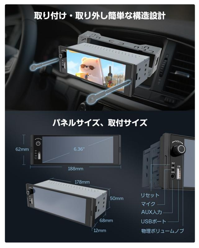
This image provides practical installation information. The top section shows the simple mechanism for installing and removing the EONON X3UJ unit using included keys. The bottom section provides precise dimensions of the unit: 188mm width, 62mm screen height, 178mm body width, 50mm body height, 68mm depth, and 12mm screen thickness, aiding in pre-installation checks.
