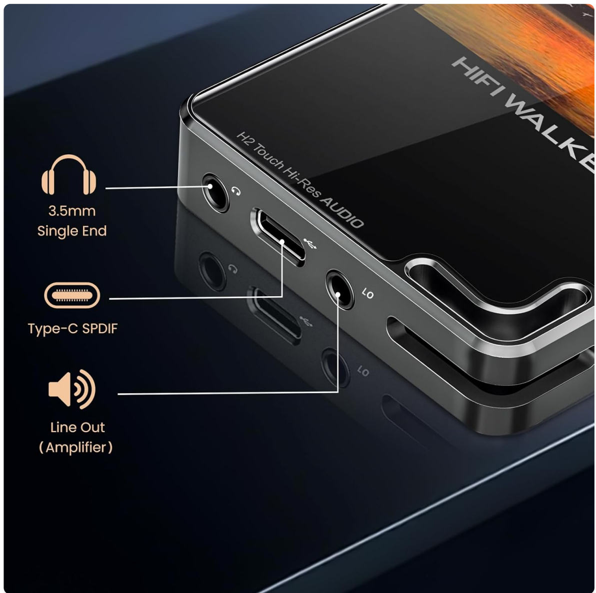
Image: Detailed view of the bottom edge of the HIFI WALKER H2 Touch, illustrating the 3.5mm single-end headphone jack, Type-C SPDIF port, and Line Out (LO) port.
