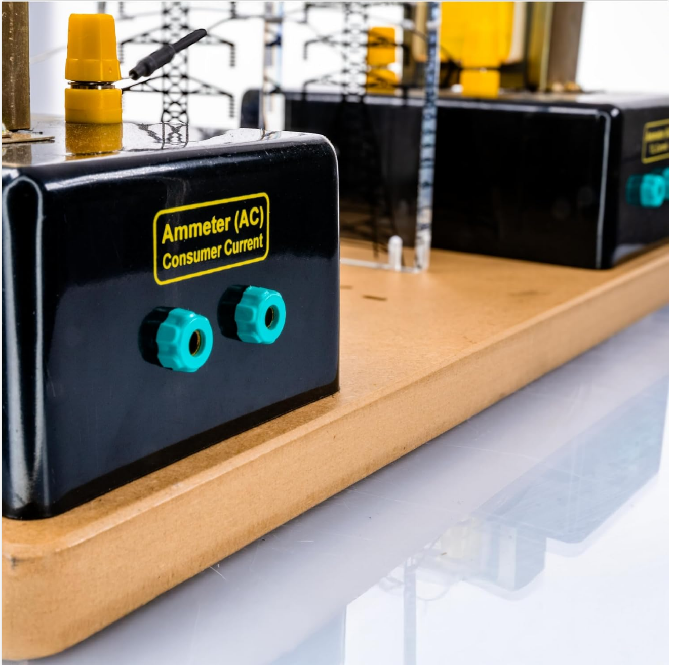
Figure 2: Close-up view of the Ammeter (AC) Consumer Current terminals. These green terminals are used to connect an external AC ammeter in series to measure the current flowing to the consumer load.
