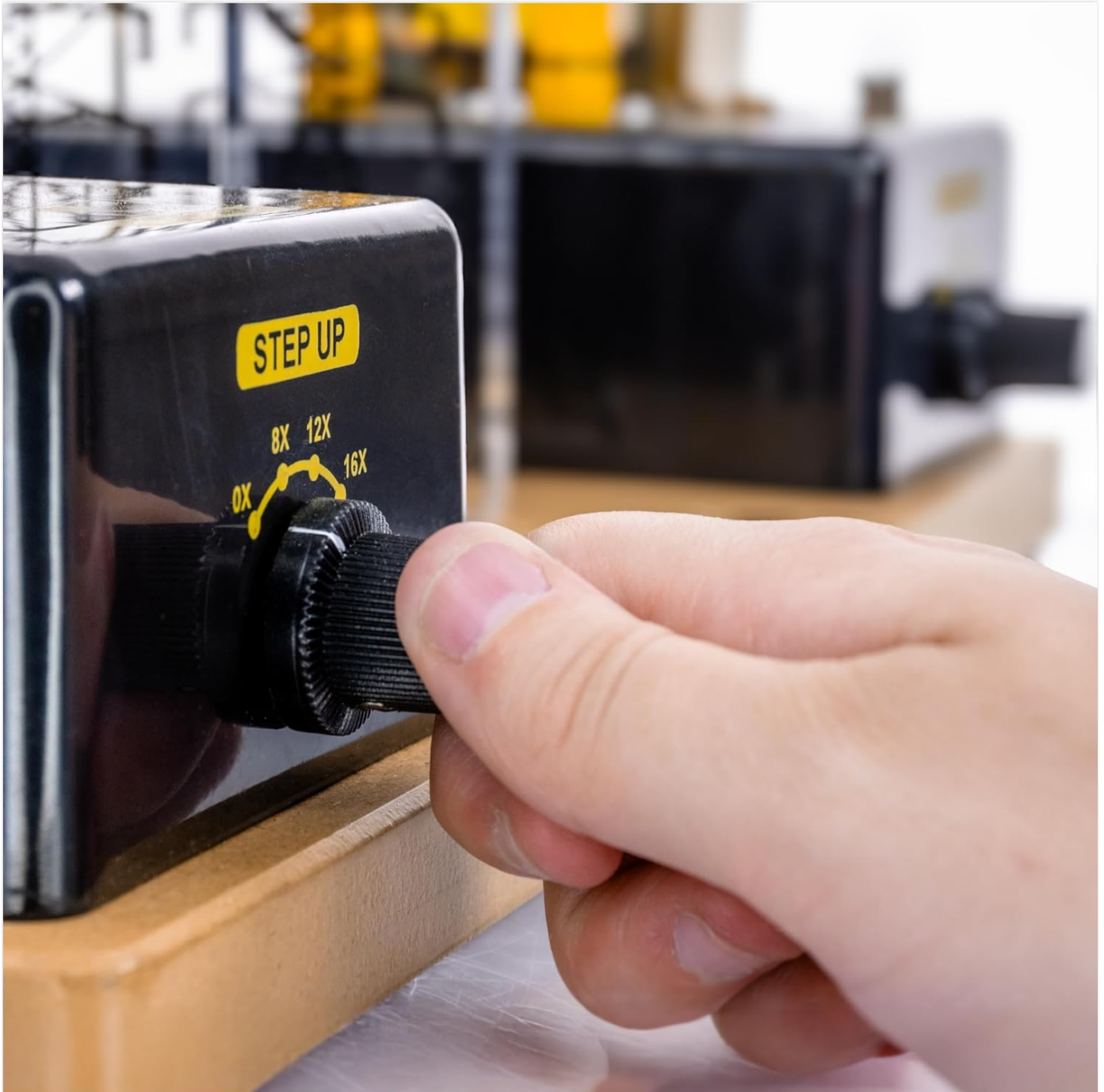
Figure 4: A hand adjusting the "STEP UP" knob on the left side of the apparatus. The knob allows selection of voltage multiplication factors (0X, 8X, 12X, 16X) for the step-up transformer.
