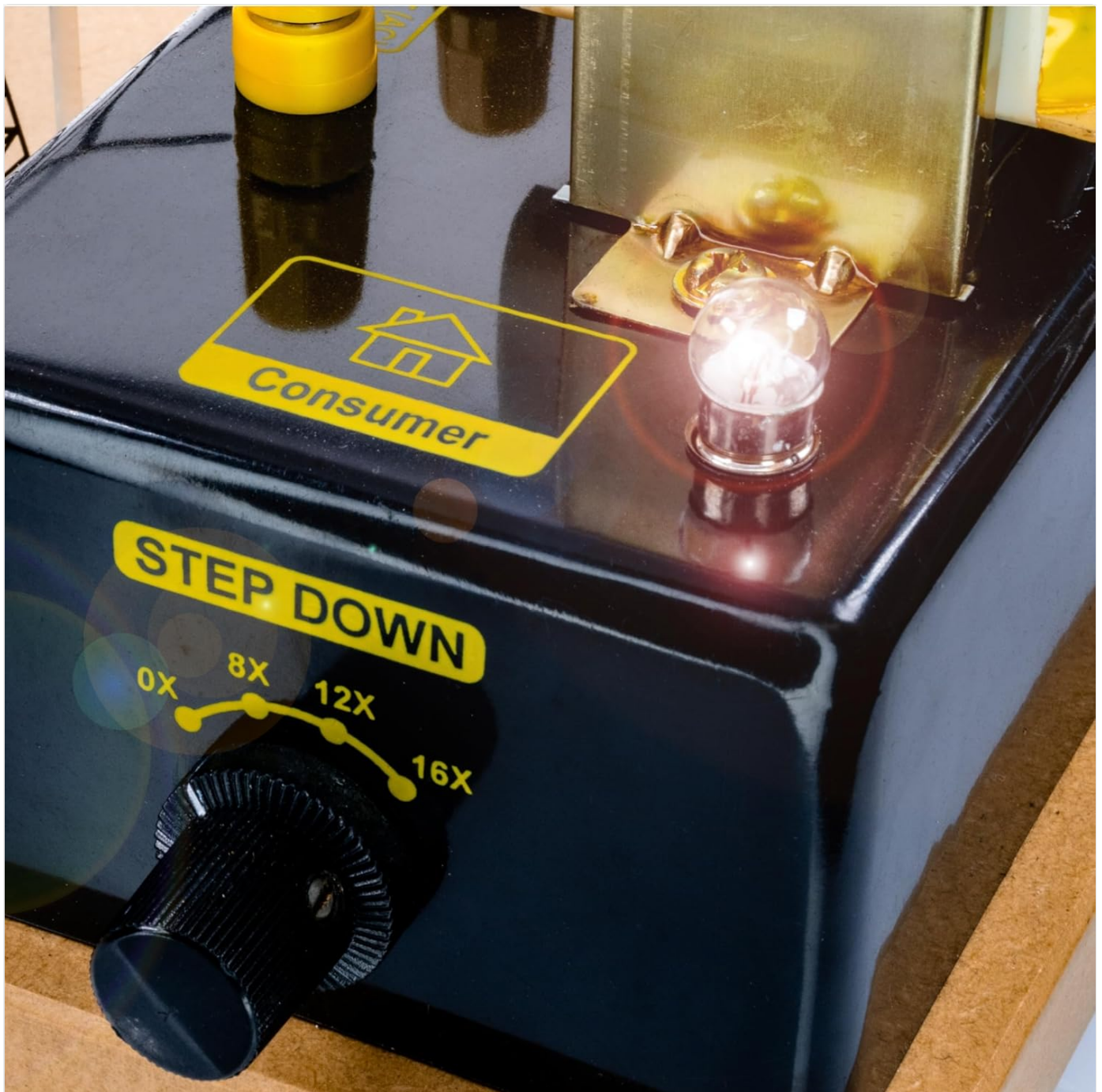
Figure 5: Close-up view of the "STEP DOWN" knob and the consumer load bulb on the right side of the apparatus. The bulb is illuminated, indicating power delivery. The knob allows selection of voltage division factors (0X, 8X, 12X, 16X) for the step-down transformer.
