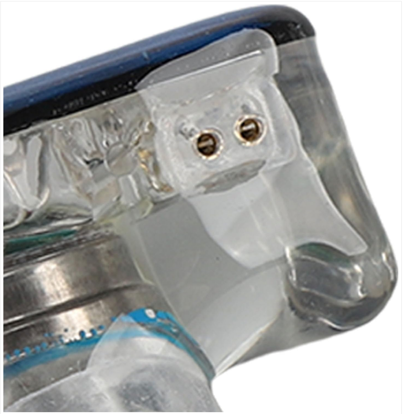
Image: A detailed view of the 2-pin connector on the earphone unit, where the detachable cable is attached.
