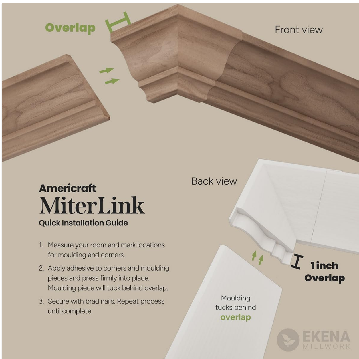
Figure 1: MiterLink Outside Corner Installation Diagram. The moulding tucks behind the overlap for a seamless appearance.
