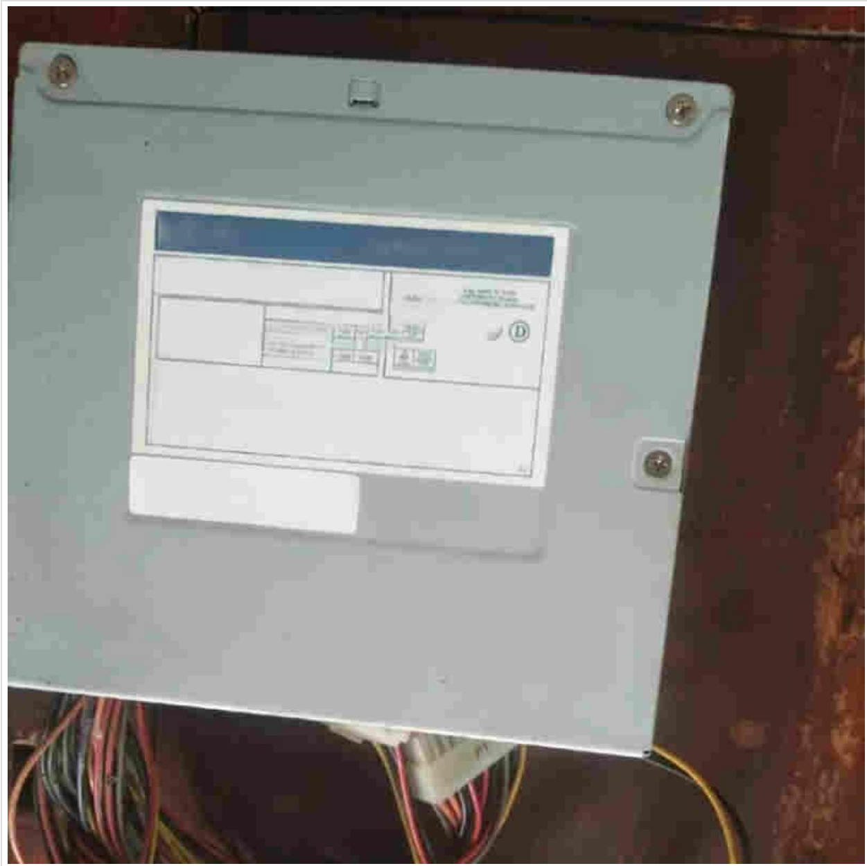
Figure 1: Front view of the Generic Industrial Computer Power Supply GPS-300AB-100V. The image shows the grey metal casing of the power supply unit with a white label affixed to its top surface, displaying technical specifications and certifications. Various colored wires are visible extending from the bottom of the unit.
