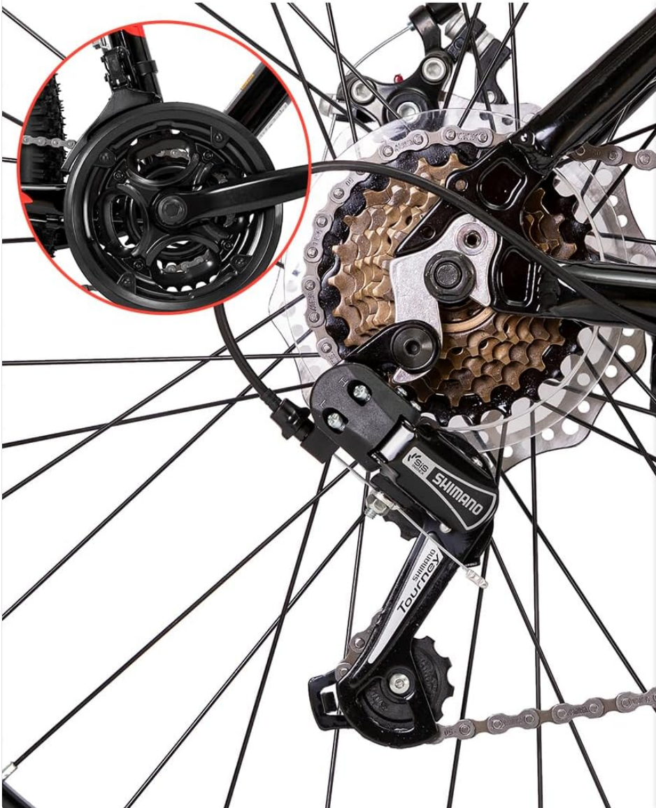
Image: Detailed view of the 21-speed Shimano rear derailleur, indicating precision shifting.
