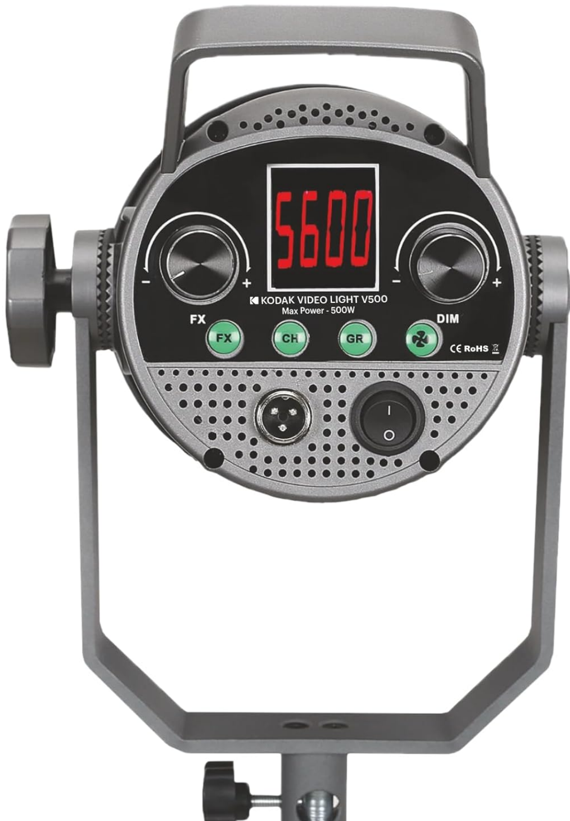
Figure 2: Rear control panel of the KODAK V500 Video Light.
