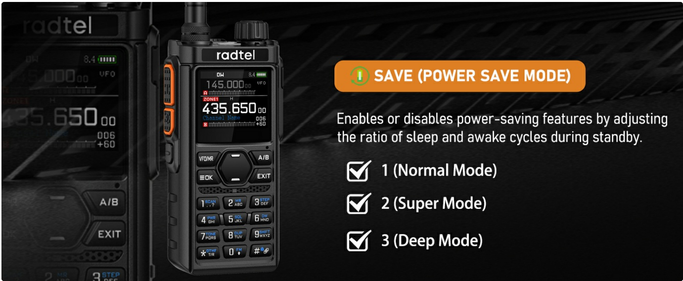
Figure 11: Power Save Mode settings to extend battery life.
