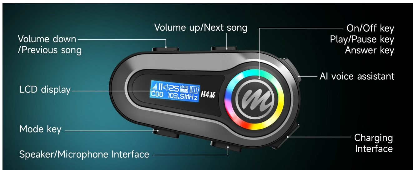
Image: Detailed diagram illustrating the location and function of each button and interface on the Moman H4M headset, including volume, power, mode, AI voice assistant, and charging port.
