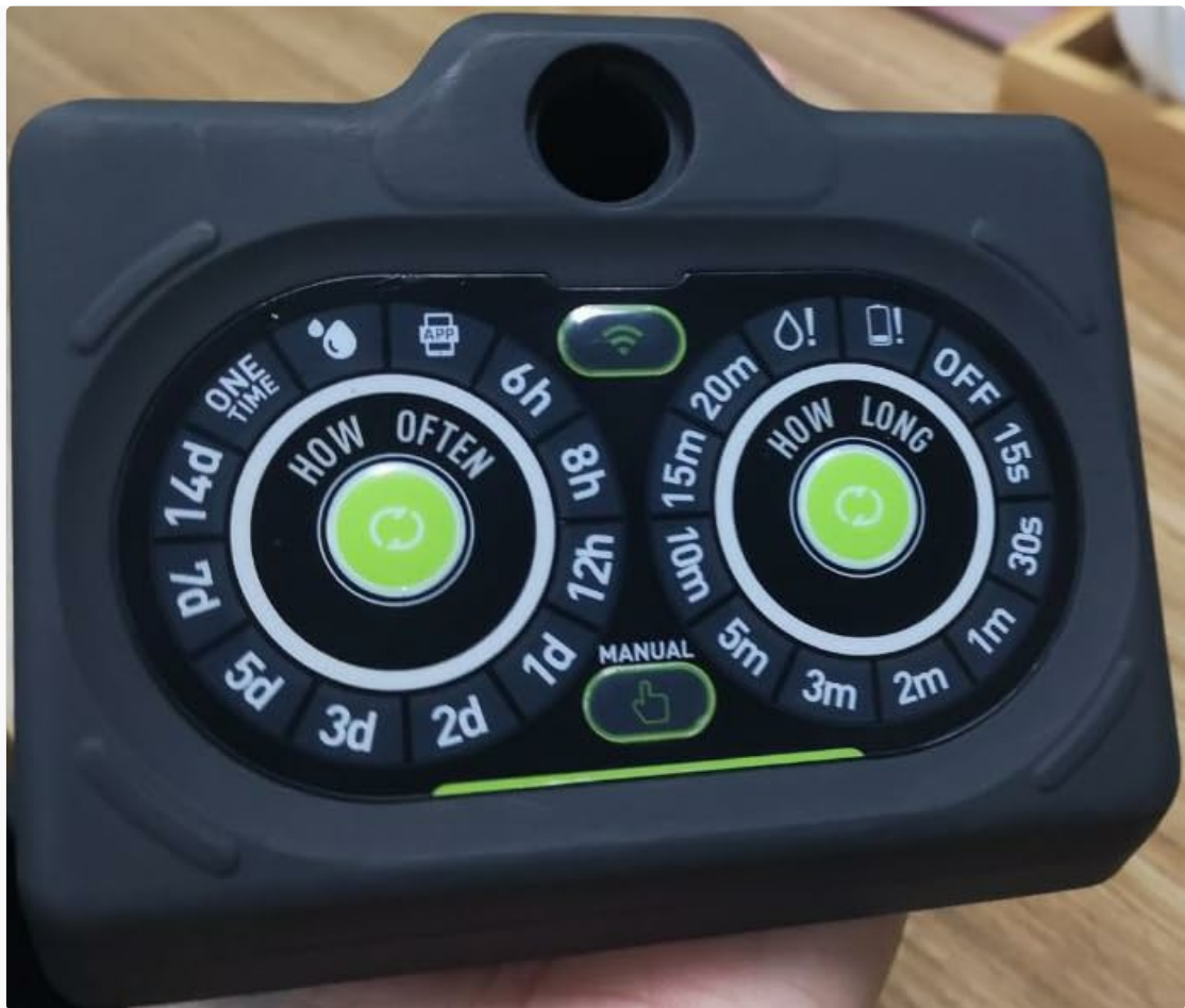
Figure 3.1: Front view of the RAINPOINT 149 controller, showing the 'How Often' and 'How Long' setting dials, along with indicators for app connectivity and manual mode.
