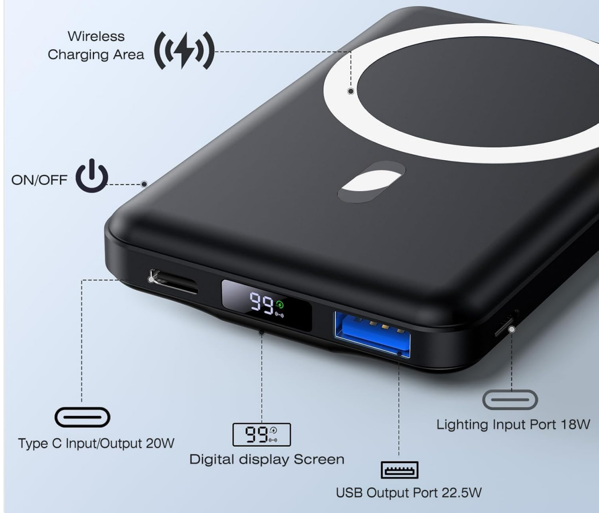
Figure 1: Overview of the AOGUERBE Magnetic Wireless Charger, highlighting the Wireless Charging Area, ON/OFF button, Type C Input/Output (20W), Digital Display Screen, USB Output Port (22.5W), and Lighting Input Port (18W).
