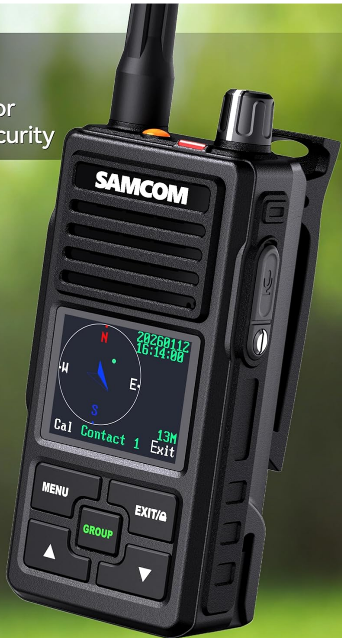
Image: Radio display showing GPS tracking settings, allowing users to set location information transmission periodically (e.g., every 30 minutes) or when a certain distance is exceeded (e.g., every 1000 meters).
