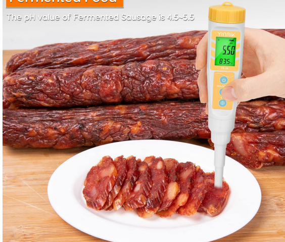
Figure 4: Measuring pH of fermented sausage. The pH value of fermented sausage is typically 4.5–5.5.
