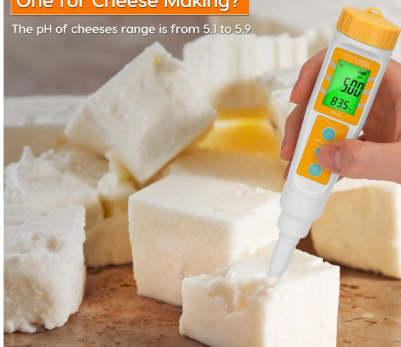
Figure 5: Measuring pH of cheese. The pH range for cheeses is typically 5.1 to 5.9.
