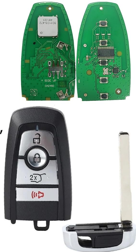
Image 3.1: Key Fob specifications including internal components and key blade.
