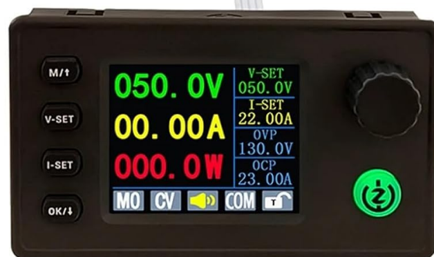
Figure 3.1: Overview of the ZK-10022 module highlighting key specifications like input/output voltage, current, and power.
