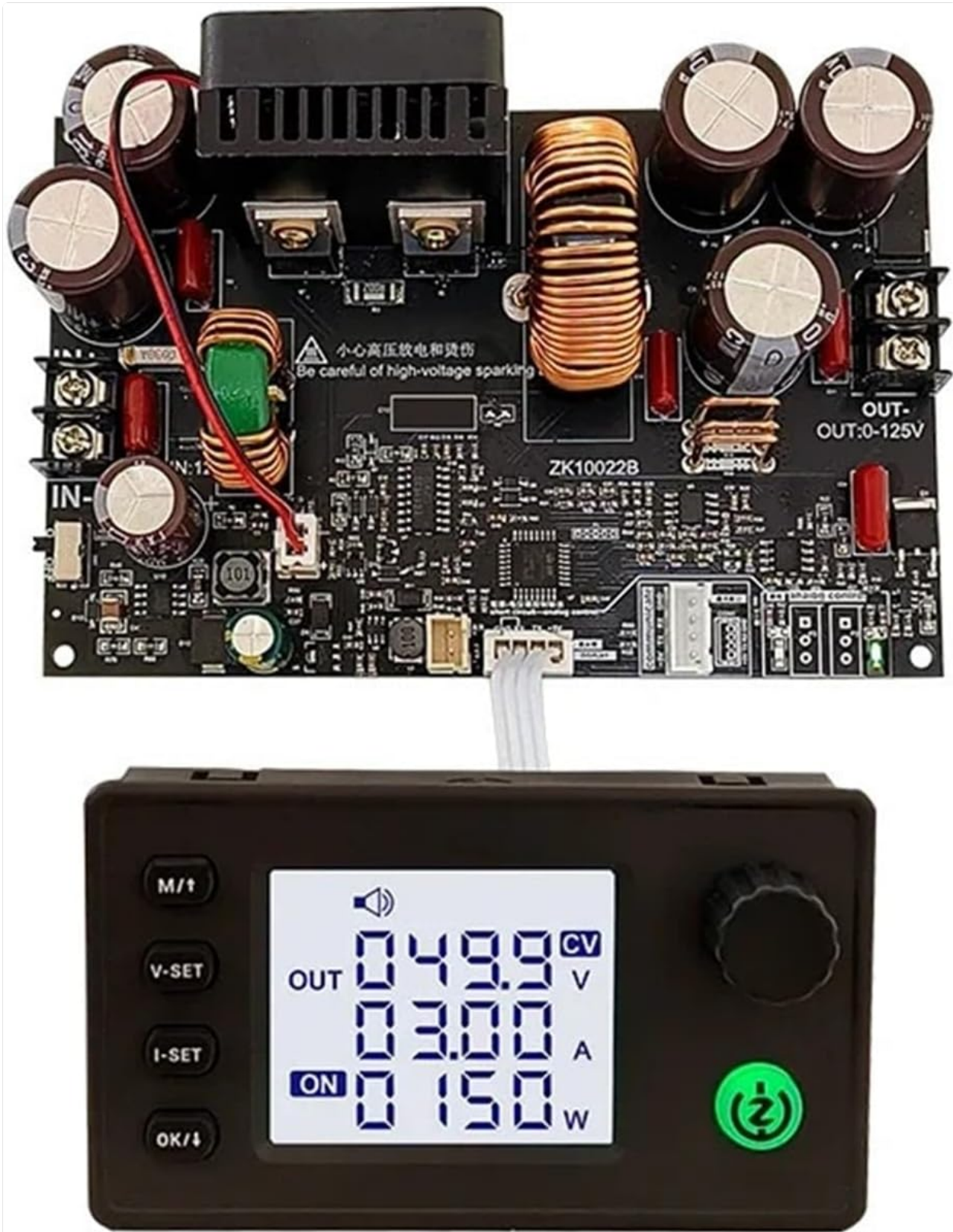
Figure 5.2: Assembled ZK-10022 CNC Step-Down Power Supply with the main board and LCD display module connected.
