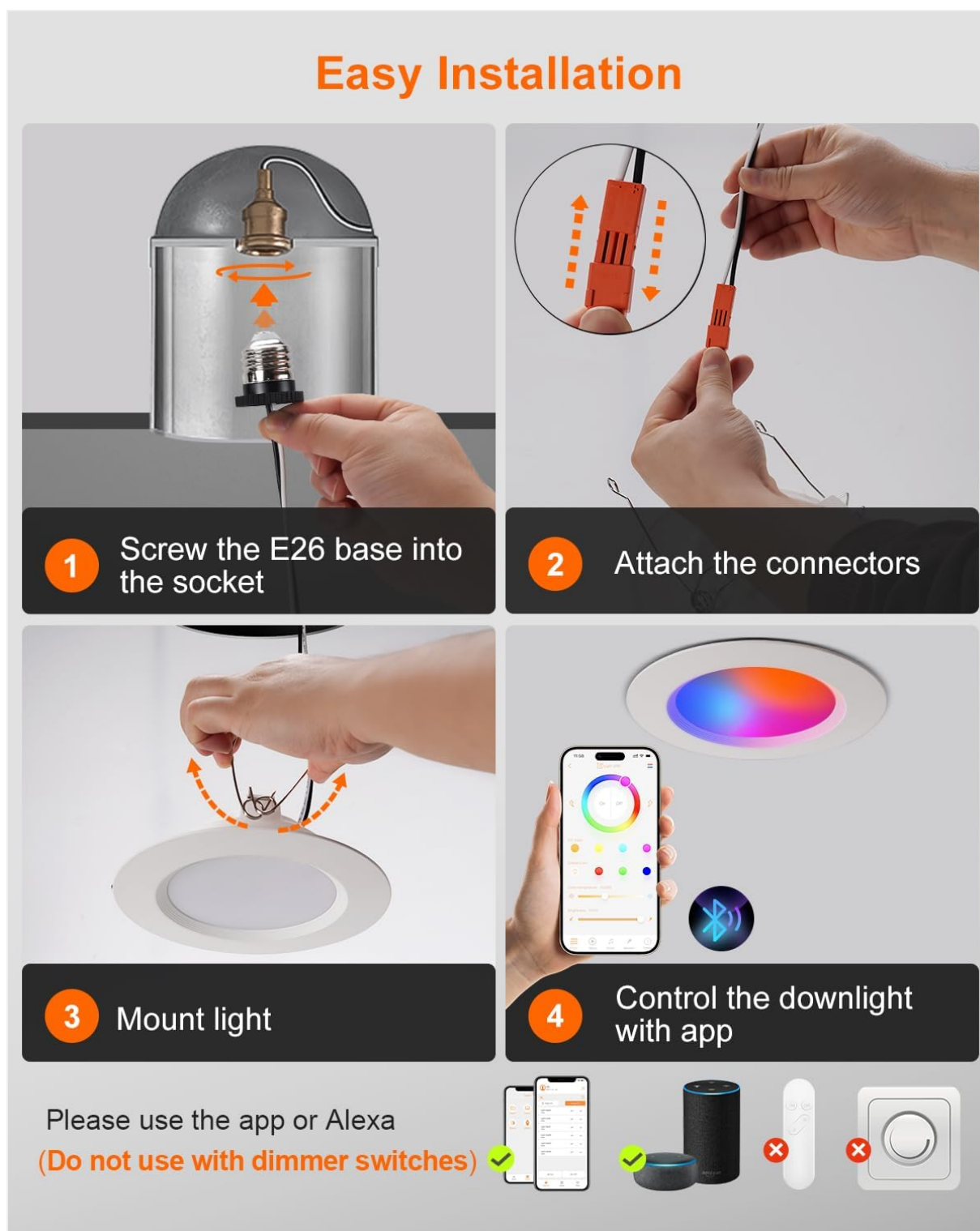
Figure 6.1: Step-by-step installation guide for DUSKTEC Smart Recessed Lighting.
