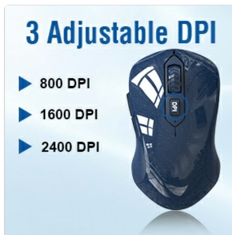
Image 3.3: The mouse features 3 adjustable DPI levels: 800, 1600, and 2400.
