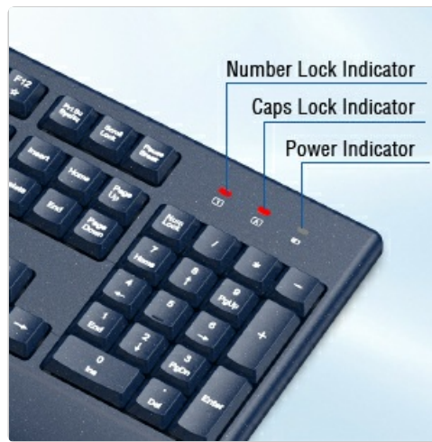
Image 3.2: Close-up of the Number Lock, Caps Lock, and Power indicator lights on the keyboard.
