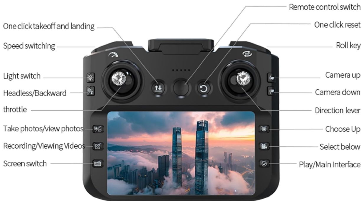
Figure 5: elecci K200 Max Screen Controller Layout.
