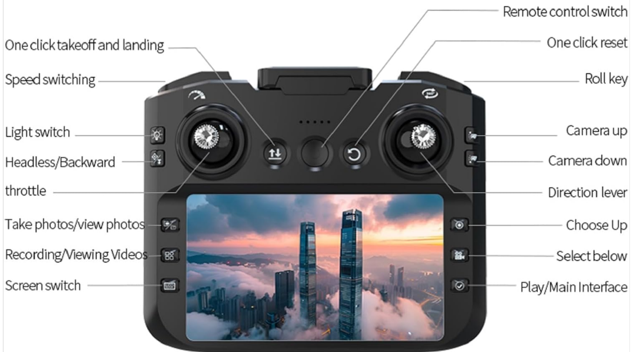
Figure 3: Detailed layout of the remote control with labeled functions for the elecci K200 Max Drone.
