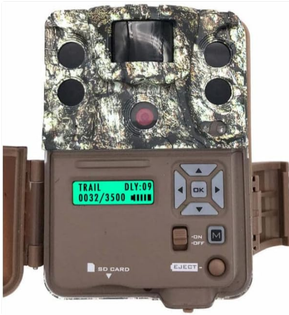
Figure 2.2: Interior view of the Browning Command Ops Elite 20 trail camera with the front cover open. This image displays the internal LCD screen, navigation buttons (OK, Up, Down, Left, Right), mode switch (ON/OFF/M), and the SD card slot with an eject button. This panel is used for configuring camera settings and reviewing captured media.
