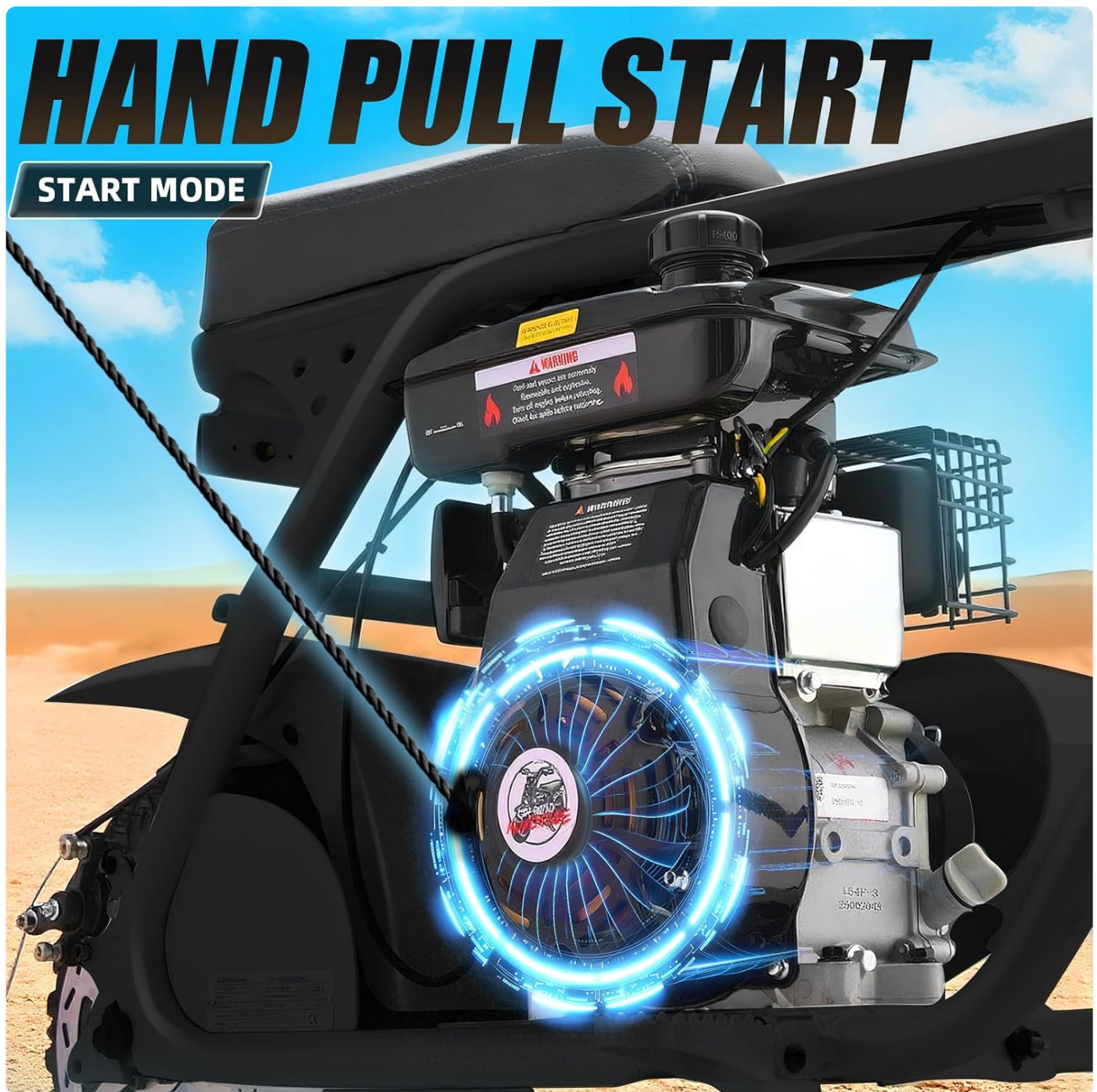
Figure 3.1: The hand pull start mechanism for initiating engine operation.
